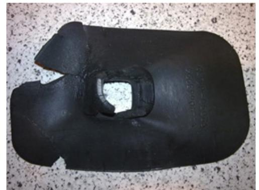
The original rubber flexible boot that fit around the clutch lever became hard and cracked over time.
